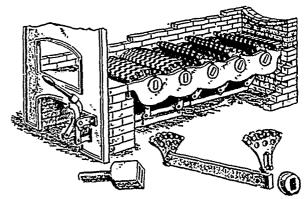
under conditions of unusual severity, has demonstrated their efficiency and durability, and the recent changes in design, tending to greater strength, enable them to promise even more satisfaction in the future. The grate is composed of a series of replaceable leaf castings, a best quality wrought iron cross bar, protected from the heat, and durable bearings in which, it is claimed, friction is reduced to a minimum. Frames for seven sections and under are made without truss.
