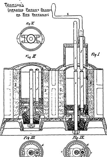
Particular care is taken in having a good mixture of iron, ensuring good sound castings. All the latest improvements in the manufacture of cast-iron pipes are adopted, one of which is the patent "beader" invented by Mr. Thomson of this firm. The pipes being cast on the ramming stool ensures the metal being of uniform thickness, which is of the utmost importance in castings of this kind. The firm has lately been reconstructed, and is now called The Gartshore-Thomson Pipe and Foundry Co., Ltd.
