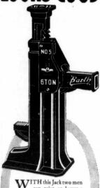
can raise or lower a load of 6 tons (12,000) lbs., a distance of 11 inches in less than one half minute. Ask your dealer for the Jack. Ask us for the catalogue. BARTH MFG. CO. 154 L St., Milwaukee, Win
