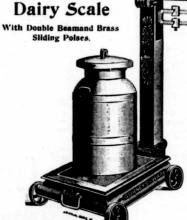
This Scale has a double beam with 100 lbs. on each bar. It is much used for weighing milk, the tare o' the can being taken by one of the poises and the other poise left free for weighing the net amount.
