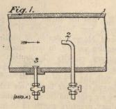
otherwise, a certain pressure, known as velocity pressure, is set up in the Pitot tube, because some of the momentum of the impining air is destroyed by the quiescent air in the tube. It has been shown by Lord Rayleigh and confirmed
