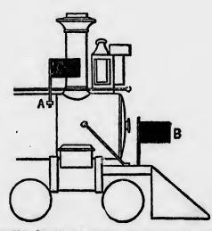
Locomotive Running Backward by Day without Cars, or Pushing Cars, and carrying Signals for Train following.
