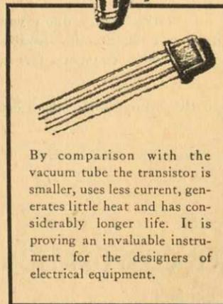
By comparison with the vacuum tube the transistor is smaller, uses less current, generates little heat and has considerably longer life. It is proving an invaluable instrument for the designers of electrical equipment.
