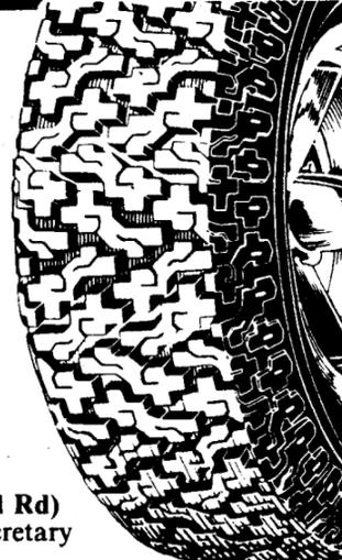
Unique jigsaw tread pattern goes through mud and snow, performs well in icy conditions. 2 belts of steel over 2 radial plies of polyester.
