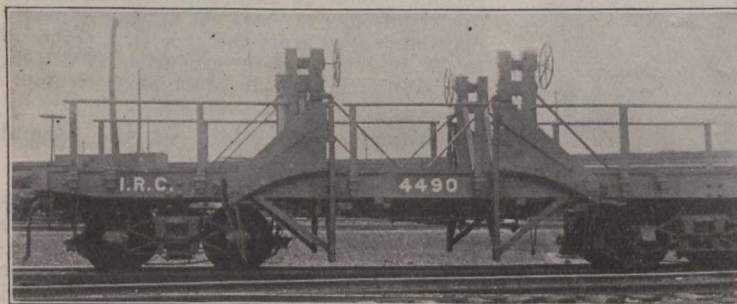
Fig 1. Ballast Trimmer with Knives Fastened up and Ready to go out on Line.
