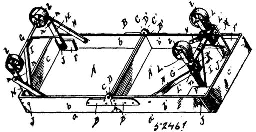
boxes, the V-shaped braces, the caster-wheels the flat springs pivoted to said boxes and the studs on said rectangular frames with which said springs engage, substantially as described.
