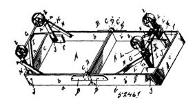
boxes, the V-shaped braces, the caster-wheels the flat springs pivoted to said boxes and the study on said rectangular frames with which said springs engage, substantially as described.
