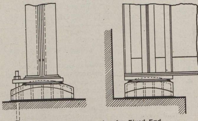
Fig. 3.—Disc Bearing for Fixed End.
