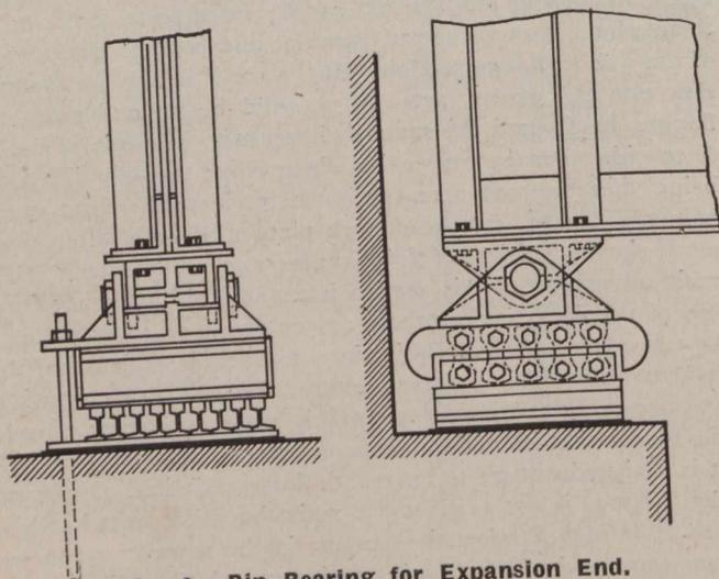
Fig. 2.—Pin Bearing for Expansion End.
