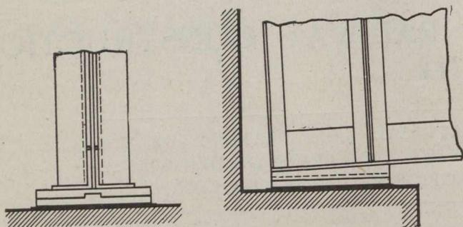
Fig. 1.—Sliding Bearing.
