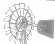
when fit ted with GRAPH-ITE bearings. They run with out oil; no more CLIMBING TOWERS TO OIL BEAR-
