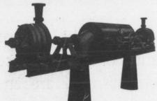
Two Worthington 3-Stage Turbine and McCormack Water Wheels, built for Port Arthur, Ont., Water Works, 1440 gal. per minute against 250 ft. head.
