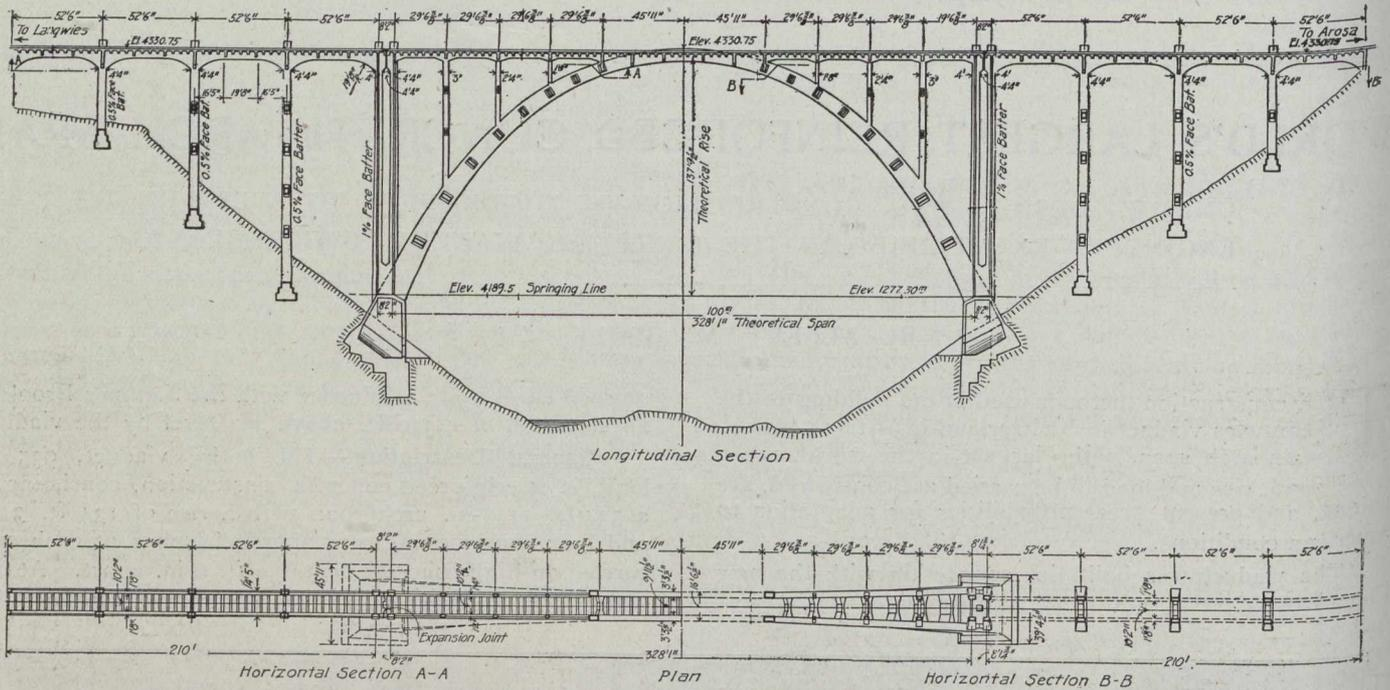
Fig. 2.—Plan and Sections, Langwies Viaduct.
