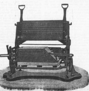
This Machine makes all blocks face down—"the only practical way"—allowing of a richer and finer facing, producing blocks that are perfect in appearance and impervious to moisture.
