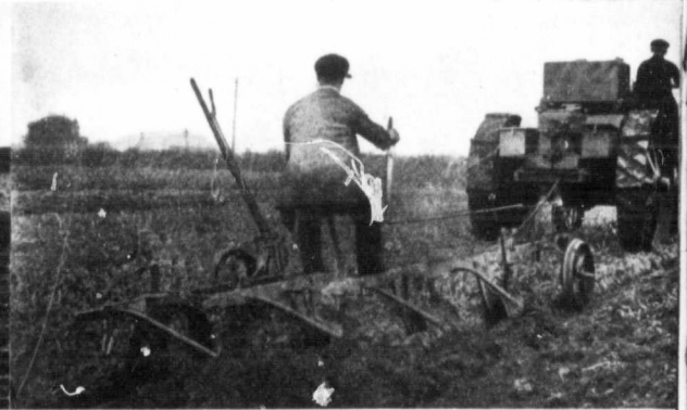
A Universal (English) Gas Tractor Plowing at a Depth of 12 inches in England.
