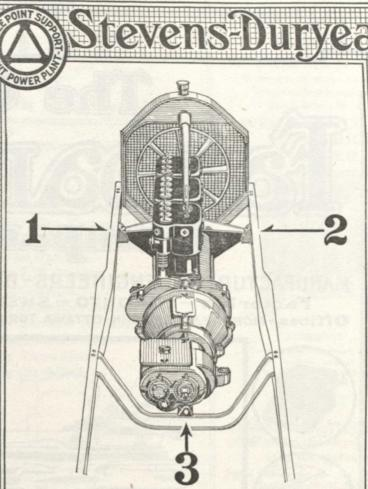
Transmission and clutch bolted directly to the engine base. That's the "Unit Power Plant". Then it is suspended at points 1, 2 and flexible point 3 - that's flexible "Three Point Support"
