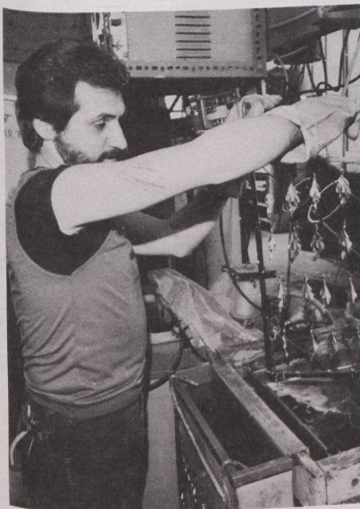
An employee gold plates jewellery at the Michele Lynn plant in Hull.
