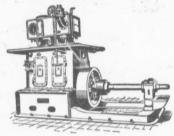
A Customer says:— "We have used one of your Vertical High Speed Engines, English Type, forced lubrication, since 1907. The Engine runs at 425 revolutions per minue almost constantly night and day. It has given us every satisfaction and so far has cost us nothing for repairs."
