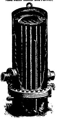
GREAT EFFICIENCY, SIMPLICITY OF CONSTRUCTION and LOW COSL Has a Cast Iron shell, which will never wear out, with seamless drawn brass tube expanded into tube-plates at top and bottom, with double blow-off.
