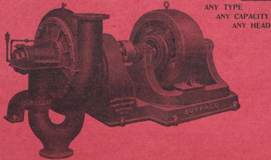
8 inch Double Suction Turbine Pump and 85 H.P. Variable Speed Motor, 900 to 1000 R.P.M. 800 to 1800 Gals. per minute against 115 feet total head.
