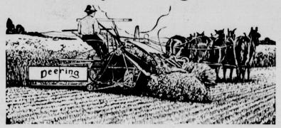
HE main frame of the Deering New Ideal binder is made of tough, strong steel bars, hot-riveted together, forming a unit which the hardest usage cannot twist out of shape. Ball and roller bearings make the machine light running. The reel is strongly braced and can always be held parallel with the cutter bar whether working high or low. The reel is easily adjustable to the right height for handling different stands of grain.
