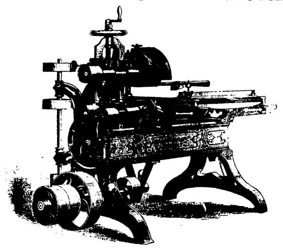
The above cut represents our No. 1 Tenoning Machine, with Double Cutter Heads. It weighs 1300 lbs., and cuts 8 inches at one cut, or 10 inches at two cuts.
