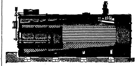
IS PORTABLE. Has an outer casing and requires no brickwork.
