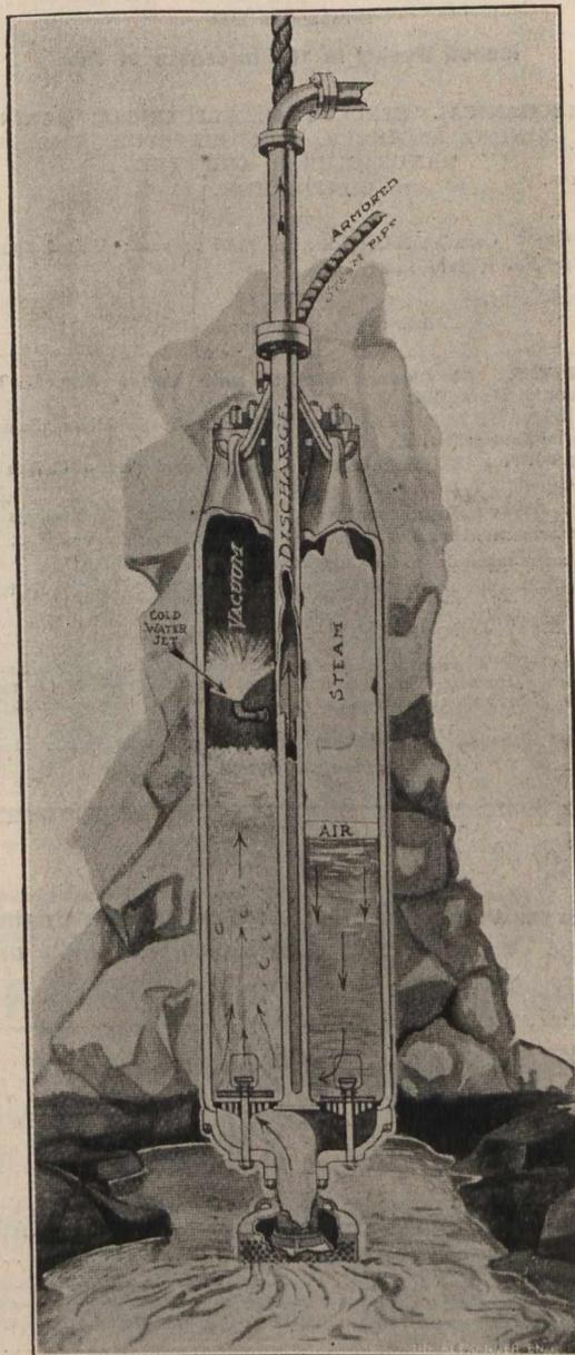
thing which moves, except the four round rubber valves, two in the suction and two in the discharge pipes. Thus the gritty material can be handled without the necessity of frequent repairs because the Emerson pump employs no plungers, pistons, piston rods, glands, stuffing boxes nor any other moving parts come in contact with the water being pumped.
