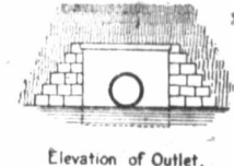
Elevation of Outlet.
