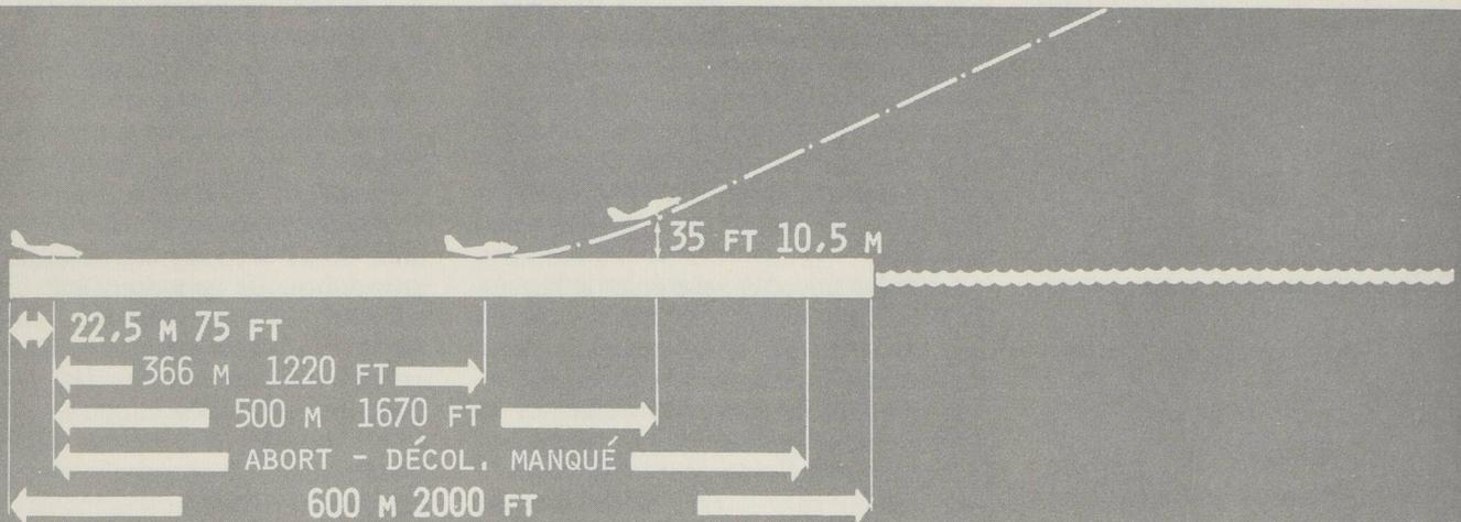
THESE DIAGRAMS ILLUSTRATE THE DHC-7 OPERATING FROM A 2,000 FOOT DOWNTOWN STOLPORT AT A REPRESENTATIVE GROSS WEIGHT OF 36,000 LB. MAXIMUM TAKEOFF WEIGHTS FOR OPERATION FROM A 2,000 FOOT STOLPORT AT SEA-LEVEL, ZERO WIND; RANGE FROM 37,400 LB AT 59°F TO 36,000 LB AT 90°F.
