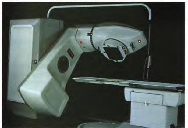
Head rotation on Theratronics cobalt 60 radiotherapy treatment units permit treatment set-ups that are not possible on accelerators.
