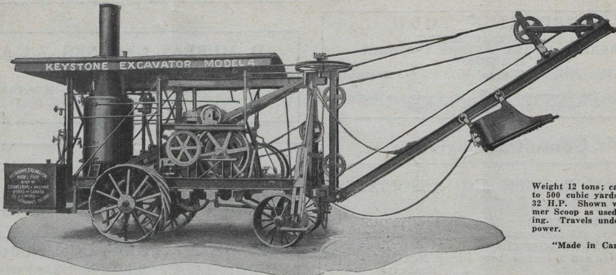
Weight 12 tons; capacity 300 to 500 cubic yards per day; 32 H.P. Shown with Skimmer Scoop as used for grading. Travels under its own power.
