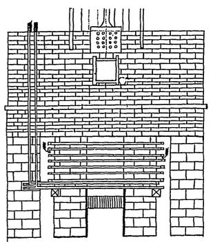
burned in five years, some in ten years; the only four we have left now working are those in the cottages A and B I made 27 years ago. The two pipes, flow and return, are laid around in recesses against the outer walls and partitions above the baseboards; they have been in the main building for nearly 50 years. and in the cottages for 32 years.
