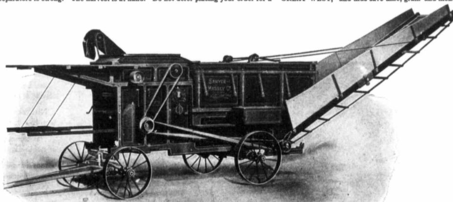
The Little "Eclipse" Separator—30" Cylinder, 36" Body
