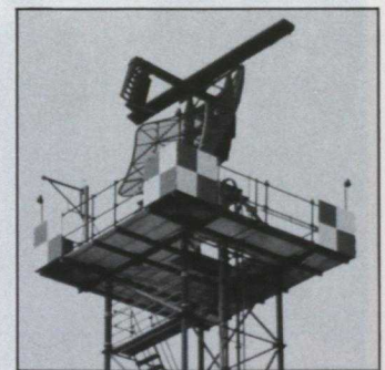
ASR-910 airport surveillance radar
