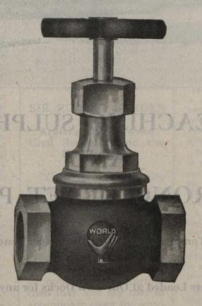
Especially recommended for all-round valves and suitable for all purposes in which a valve can be used from the lowest to the highest pressures of steam, gas, air, water or oil. A special feature of this valve is the "DOUBLE TAPER SEAT," enabling valve to be re-packed when open and under full pressure of steam
