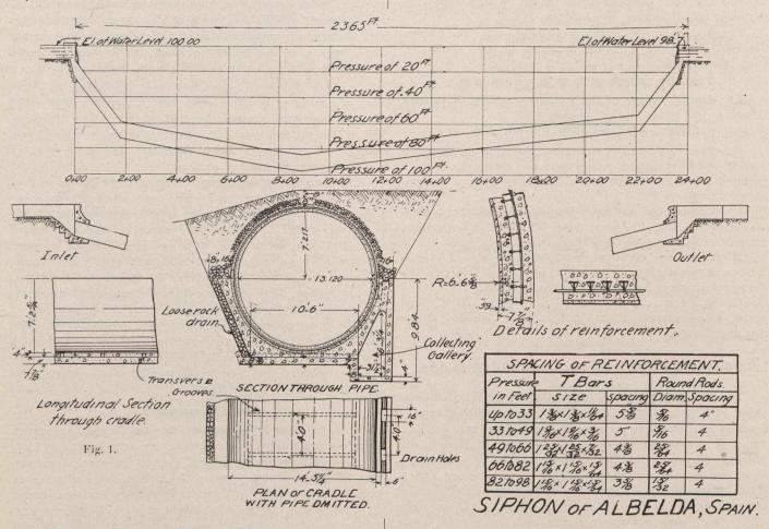
conduit would find an easy passage into the drains. The concrete used consisted of about 1 part of cement to 41/4 of sand and 81/2 parts of gravel passed through a 23/4-inch screen.
