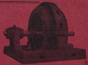
2000 KW. Westinghouse Water-Wheel Alternator
