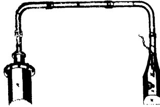
3204 Bourgeois' Attachments to Pumps for Pumping Sand, Gravel, &c.
