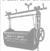
Double Purchase makes the Beatty Carrier lift with half the power. The Beatty will tip to either side to discharge.
