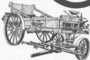
You can only buy one manure spreader with the Reversible, Self-Sharpening, Graded Flat-Tooth Cylinder—and that is the Genuine Kemp. Because of this Graded Flat-Tooth Cylinder the Genuine Kemp is at least one-third lighter draft than any other spreader.
