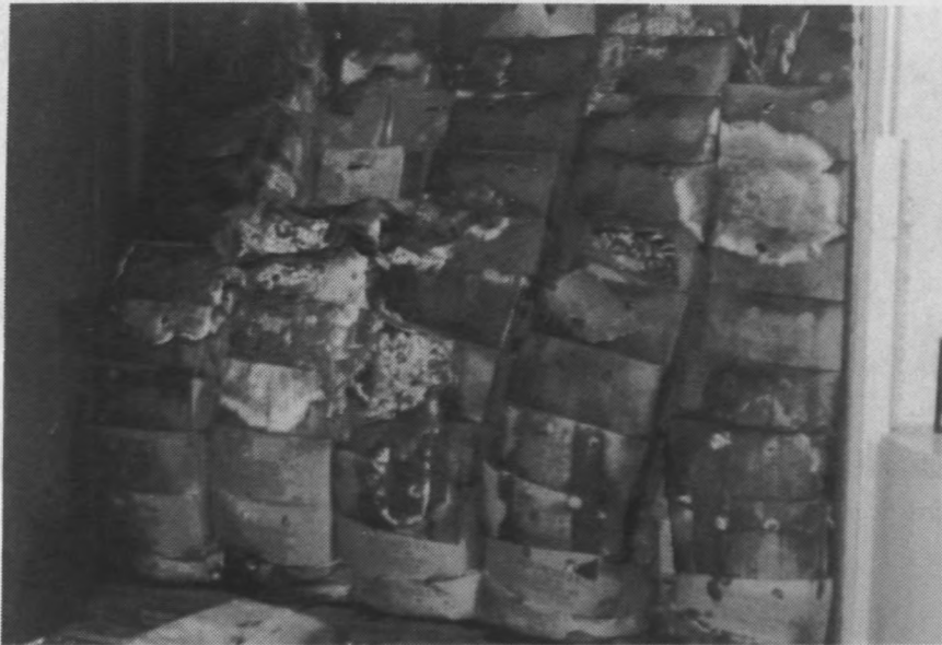
Too tight a stow, no separations, container leaked causing water damage.
