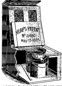
INUDOROUS PORTABLE BEDROUM COMMODE A-Urine Separator. B-Urine Receptacle. C-Excrement Tank.
