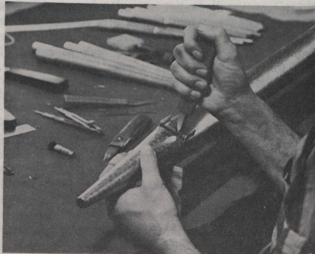
Casavant organ pipes are still made by hand as they were in the eighteenth century.
