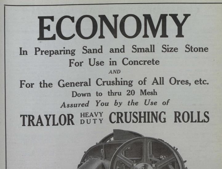
Owing to the automatic lateral shifting device, you get the maximum tonnage per set of shells and consume the minimum horse power; for all *corrugating* and *flanging* of the roll shells are eliminated by this strong, simple and positive device.
