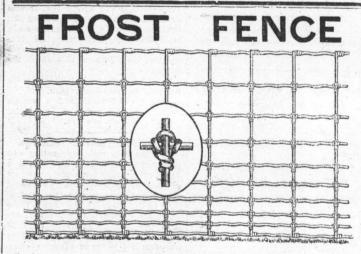
This fence is made in Canada enitrely of Canadian products. All the wires are full size true to gauge. Laterals and uprights are all No. 9 Hard Steel, well galvanized stock. Laterals are given a deep, and continuous wave for "give and take." These coils or waves serve like a spring keeping the fence tight throughout all seasons and under all conditions. It is used by the principal farmers everywhere. The cost to you is no more than the price of other fence of equal weight. Insist on getting it.
