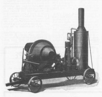
You wonder how such a simple looking machine as the "Smith" Mixer is able to produce such fine concrete. It certainly looks and is simple, but have you ever looked inside a "Smith" Drum and seen how the contents are turned over, cut away, lifted up and tumbled into a central mass many times a minute—
