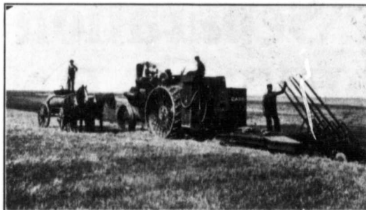
A Case 32 H.P. Steam Tractor pulling a John Deere Engine Gang.
