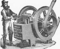
Quartz, Emery, Gold and Silver Ores, and all Hard or Brittle Substances; also for making Railroad Ballast and Concrete. Our Adjustable Toggle Block enables us to adjust the Machine while in motion to the size of any stone or particular product. There are other improvements possessed by these Machines not equalled by any other in the world. Gold Medal awarded at the Massachusetts Mechanics' Association 1881, and Silver Medal (Specia) at American Institute, N.Y., 1882.
