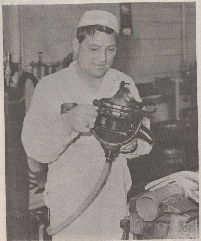
Welder Bill Dereski prepares to put on a compact and versatile welding helmet developed at the Whiteshell Nuclear Research Establishment. The helmet features a modification which permits the use of an auxiliary air supply system.
