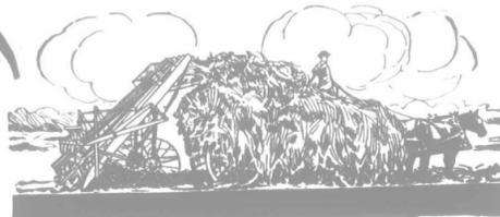
leaves because the self-expanding throat allows hay to pass freely onto wagon without wadding, tangling or jamming. An apron at top keeps hay from spilling or blowing off side of load. Wheels set underneath so it can be taken through gates and operated close to fences, can be coupled or uncoupled without crawling under wagon, uncoupled without getting off load.
