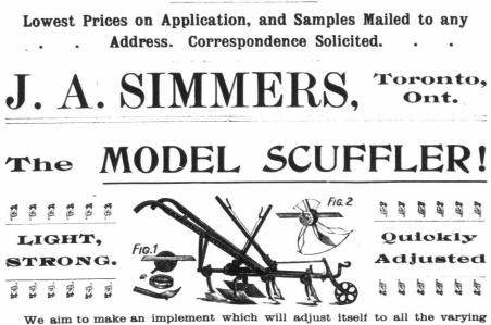
conditions of soil in the quickest possible manner, and with the least manipulation. We accomplish this by our new patented SHANK FASTENER OR CLAMP. The change is made by loosening one nut half a turn, by which operation the point can be shifted to any conceivable position. This Scuffler is, what many of our customers have already called it, "A WORLD BEATER." It is strong, durable, and of the best material and workmanship. If your local agent does not supply you, write direct to the estate of
